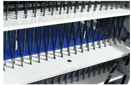
Optional automatic oil lubrication system prevents sticking of crumbs on blades. In particular recommended for slicing darker bread types.
