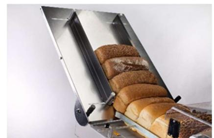
Solidly constructed stainless steel chute for extra infeed storage of up to 15 breads. Equipped with guide strips for different bread sizes. Chute can be folded down completely when not in use.
