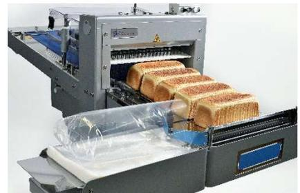
Standard equipped with high-performance bag blowing device for plastic bags.
